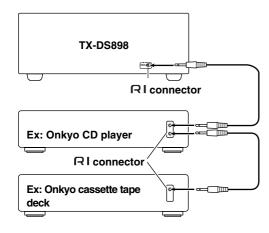
To connect components using the RI terminal, simply connect a remote control cable from this RI terminal to the RI terminal of the other component. An RI remote control cable with a 1/8-inch (3.5-mm) miniature two-conductor plug comes with every cassette tape deck, compact disc player, MD recorder, and DVD player that has an RI terminal.
